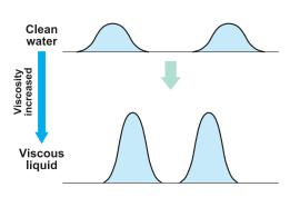
Variation in liquid flow distribution caused by increase of viscosity
