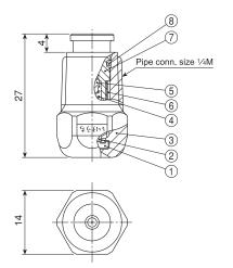
①Ceramic orifice ②Closer ③Body ④Spring (S304) ⑤Poppet (NBR) ⑥Strainer screen (S316) ⑦Strainer holder (PP) ⑧O-ring (NBR)
